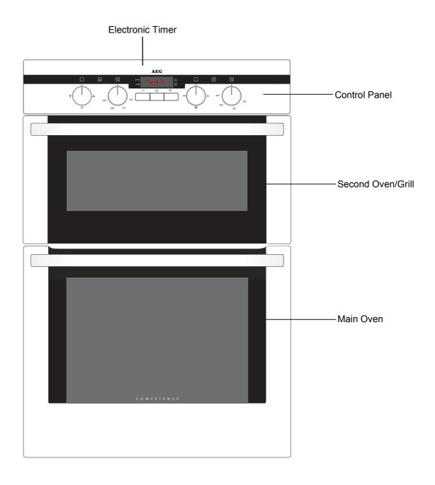
Your built-in oven comprises of a conventional second oven and dual grill in the top compartment. The main fan oven is the larger of the two ovens. It can be automatically controlled by the electronic timer.
